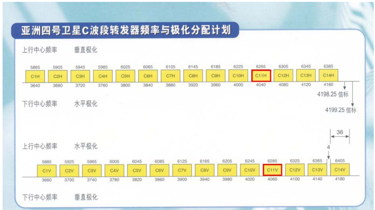
Figure 6. AsiaSat-4 Satellite Frequency and Polarization Plan
