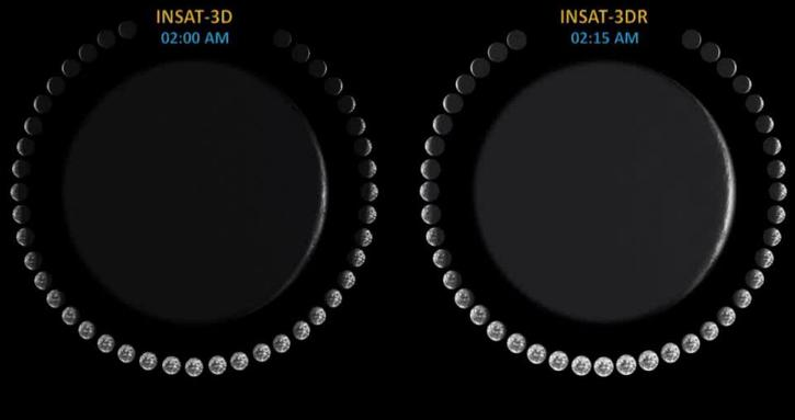
INSAT 3D and 3DR together provides observations at 15-minute interval : 48 images/day and sounding at every half an hour.
