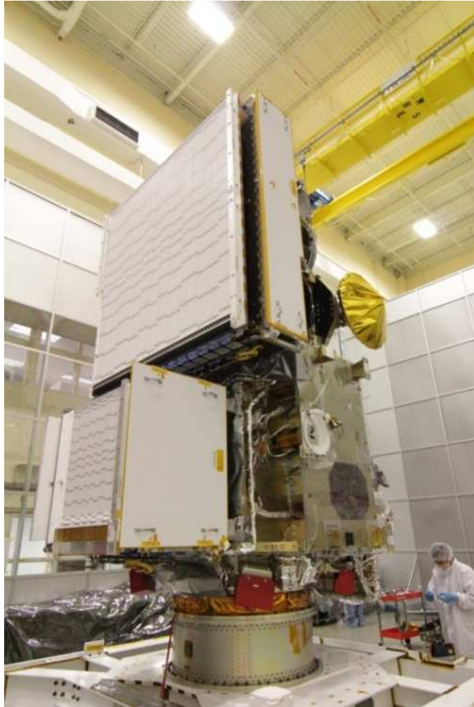
DPR mechanically integrated to the core observatory (photo provided by NASA)
