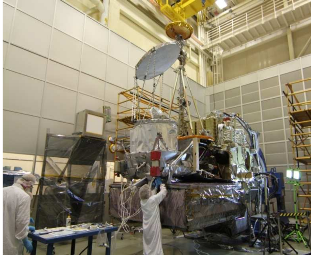
GPM core observatory in GMI and HGA deployed configuration (photo provided by NASA)
