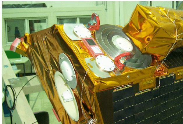
Fig. 2.2: CHAMP GPS antenna array of limb-viewing elements (left) and the zenith-looking POD antenna on a choke ring.
