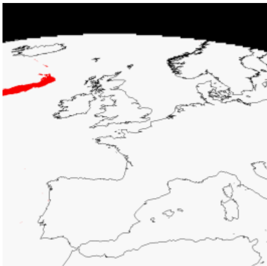
Figure 2: Volcanic ash index derived from a split-window thresholding technique also shows the extent of the ash plume, however in less detail than on the RGB above (product is for same time as Figure 1) (source: EUMETSAT)
