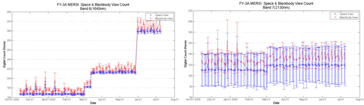
Figure 3 Scanning signal trend of space view and black body of MERSI band 4,5,6,7
