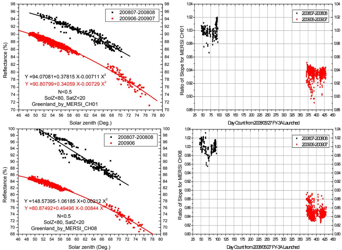
Figure 10 MERSI Calibration year-round degradation rate using Greenland observation during 2008 to 2009
