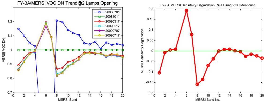
Figure 2 MERSI VOC DN at different time (left) and derived sensitivity degradation rate of 19 reflective solar bands (right)
