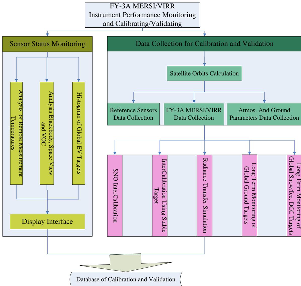
Figure 1. Optical instruments Radiance-based Calibration and Validation System Framework of FY-3A QCS
