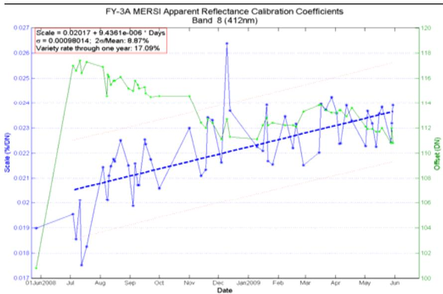
Figure 7 Calibration coefficient trend of band 8 of MERSI from site cross-calibration using Dunhuang
