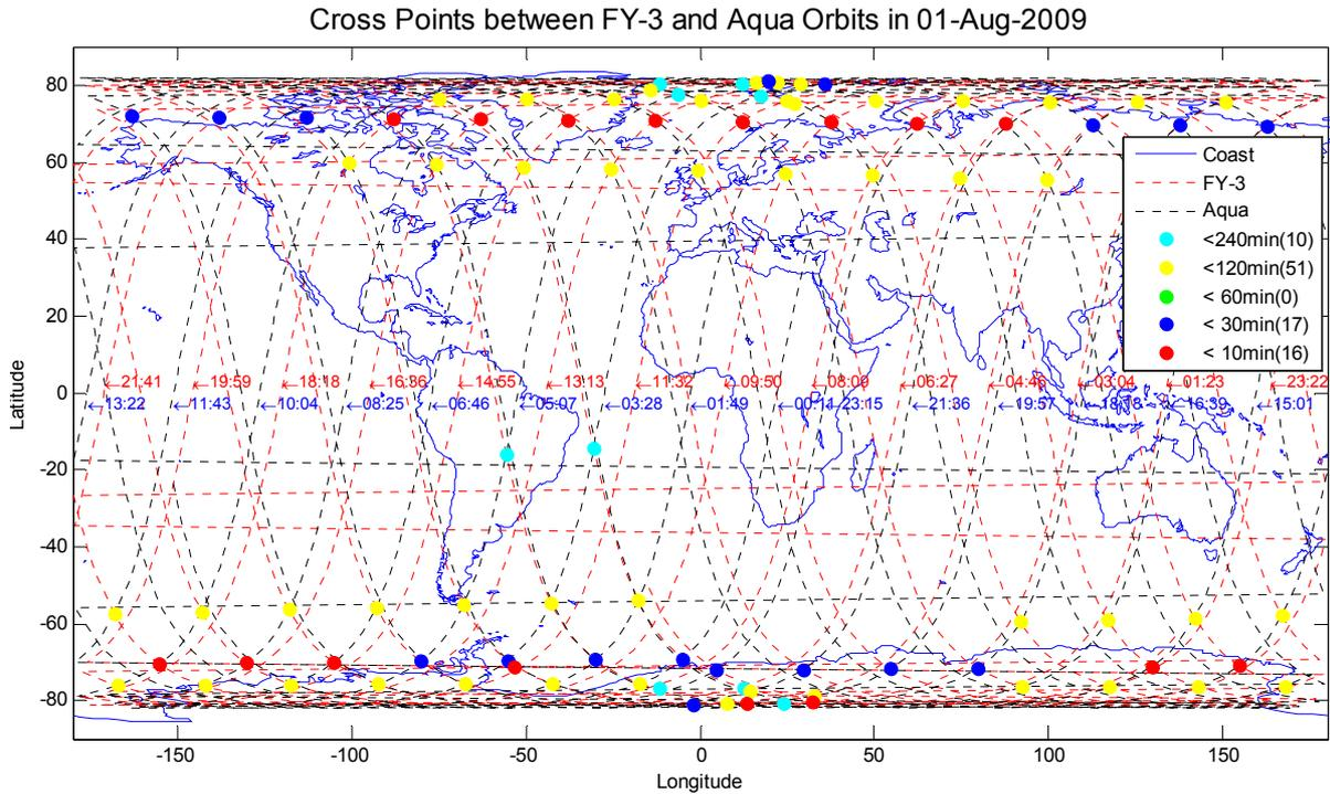
Figure 6 SNO Cross Point between FY-3 and Aqua orbit in Aug. 01, 2009
