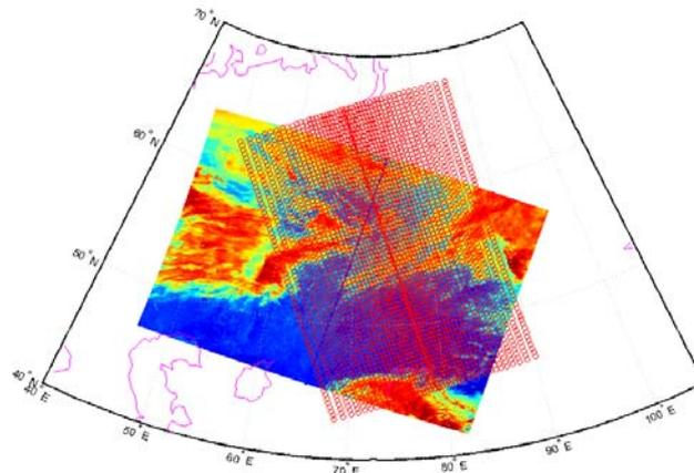
Figure4 Collocation map of VIRR(bottom image) and AIRS (overlay Grid)
