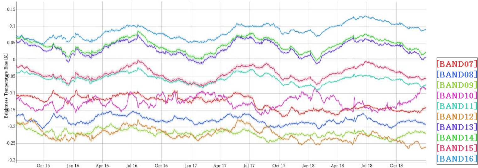
Time series of Himawari-8/AHI Tb biases w.r.t. Metop-A/IASI at std. radiance (2015-07-07 to 2018-12-31)
