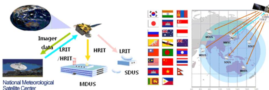
Figure 2.2: Concept of MI H/LRIT direct broadcasting
