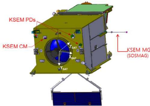
The dual magnetometer samples variations of low frequency magnetic fields at two different locations on a deployable boom to accurately measure the Earth's magnetic fields by separating the spacecraft contribution. The spacecraft charging monitor measures integrated fluxes of electrons above ~ 1 MeV that is crucial for the satellite operation. KSEM specification is as follows:
