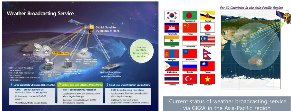
Figure 3.2 Concept of GK2A AMI UHRIT and H/LRIT direct broadcasting
