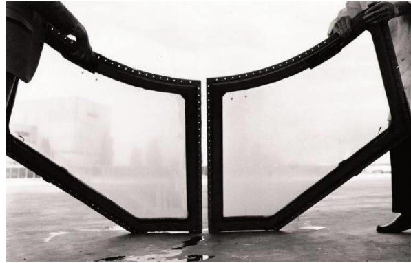
Figure 3. Damage to engine components (left) and abrasion of windshield (above) due to British Airways flight BA009 encountering volcanic ash over Indonesia in 1982
