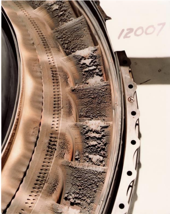
Figure 3. Damage to engine components (left) and abrasion of windshield (above) due to British Airways flight BA009 encountering volcanic ash over Indonesia in 1982
