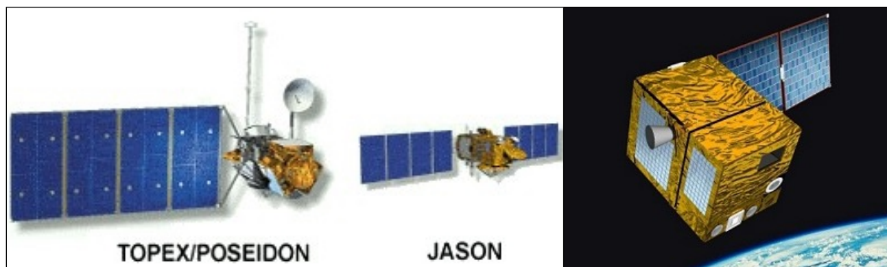
Fig. 4.5.2 - Size reduction from TOPEX-Poseidon to Jason.
