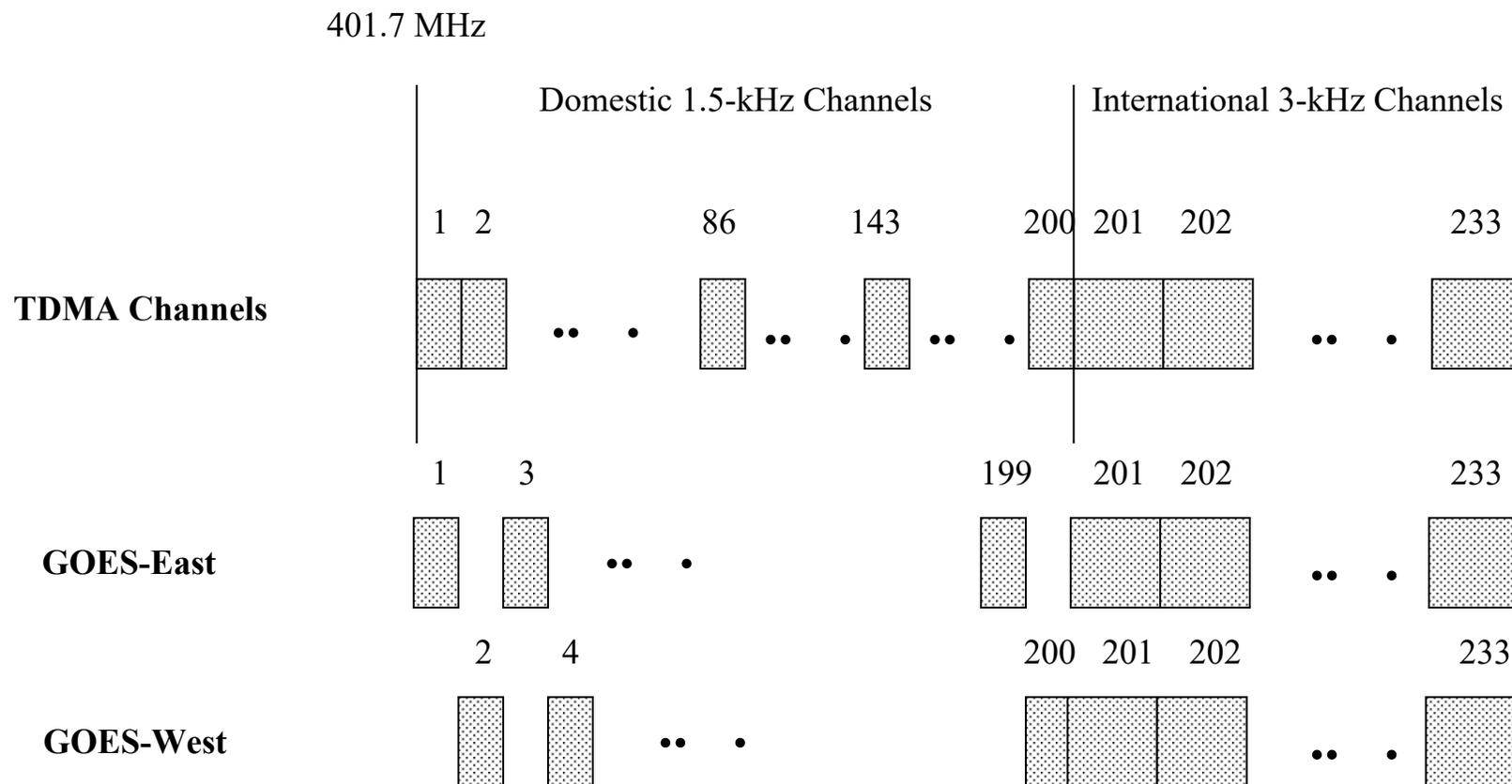
**Figure 1. GOES UHF-L Transponder's DCS Frequency Plan**
