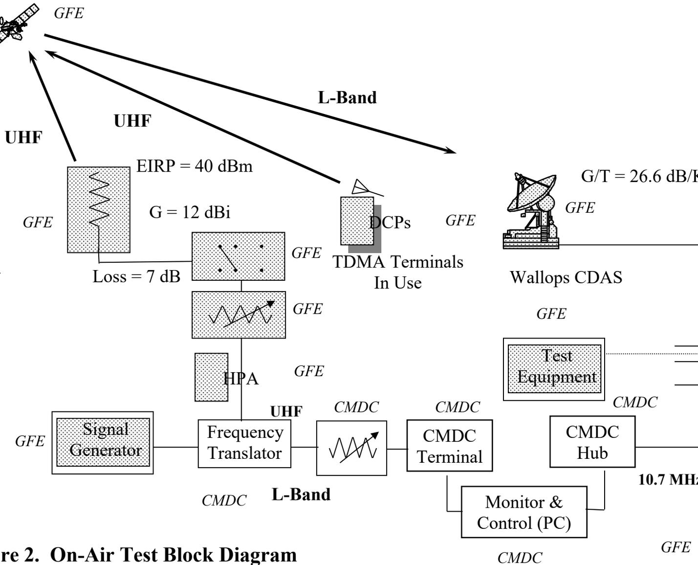
**Figure 2. On-Air Test Block Diagram**
