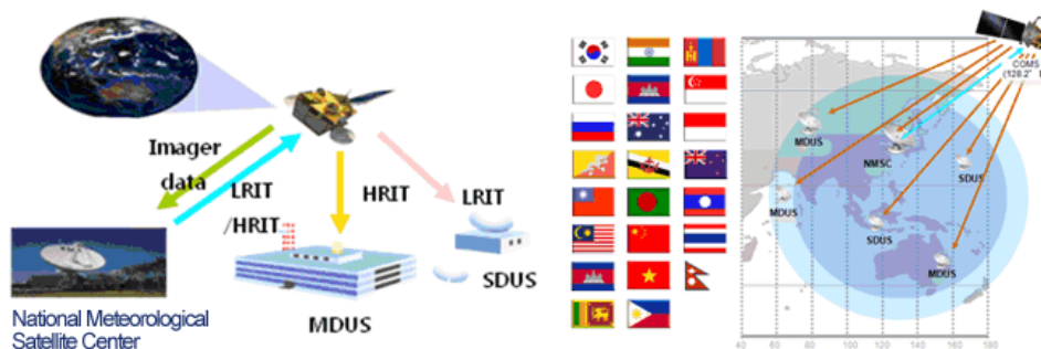
Figure 2.2: Concept of MI H/LRIT direct broadcasting
