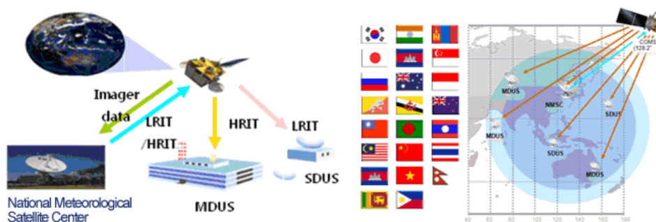
Figure 2.2: Concept of MI H/LRIT direct broadcasting
