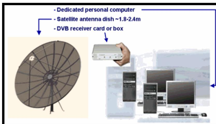
Fig. 3. Components of a typical GEONETCast Americas receiver station.
