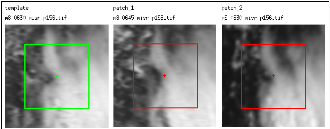
Figure 4. MPG triplet matching between Meteosat-8 HRV at 06:34 UTC (left), Meteosat-8 HRV at 06:49 UTC (center) and Meteosat-5 at 06:37 UTC (right). The template and patch windows are shown in green and red, respectively. It can be seen that there are larger differences in the cloud structures between Meteosat-8 HRV at 06:34 (left) and at 06:49 (center), due to changes within the 15-minute time interval.
