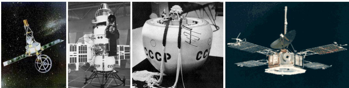
Figure 1. From the left: Mariner 2 spacecraft, Venera 4 bus with the entry probe at the bottom, Venera 4 probe showing the bridle and transmitter, and Mariner 5 spacecraft.
