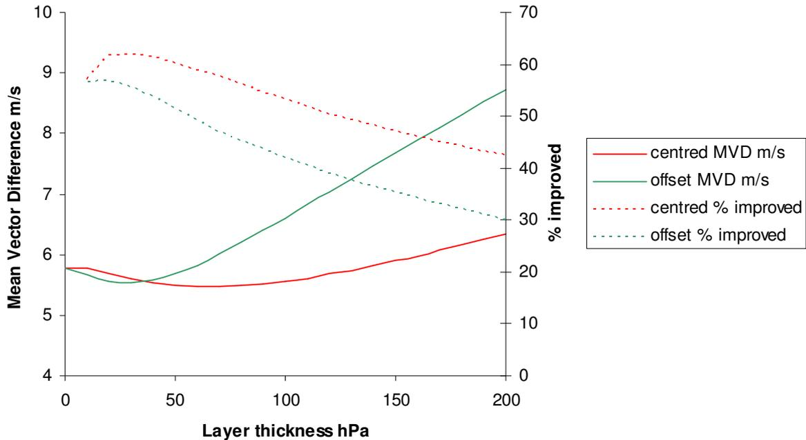
Figure 7: Preliminary results investigating improvement in mean vector difference statistics as a function of layer width for Meteosat-9 IR 10.8 AMVs valid on 16 February 2010 00z run (2100-0300 UTC).
