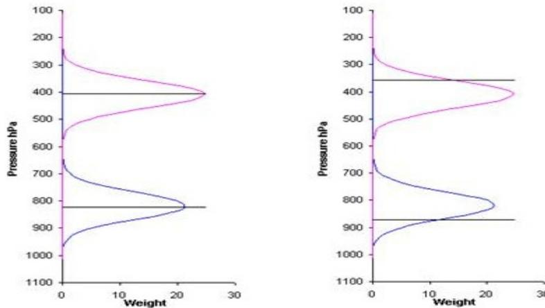
Figure 6: Examples of Gaussian layer operators (left) centred and (right) offset.
