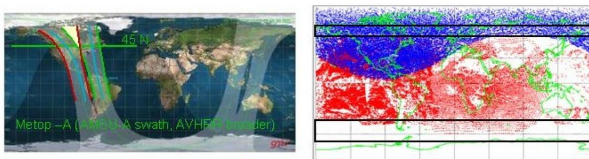
**Figure 2:** (left) Example of improved coverage using image triplets from alternate Metop-A/B overpasses (Metop-A highlighted in green and red, Metop-B in blue). The yellow triangle shows the overlap between the three overpasses (area where AMVs can be produced with image triplets). Using only image pairs would provide coverage globally. (right) Example coverage from one satellite in highly elliptical orbit (blue) - from Riishojgaard, 2006.
