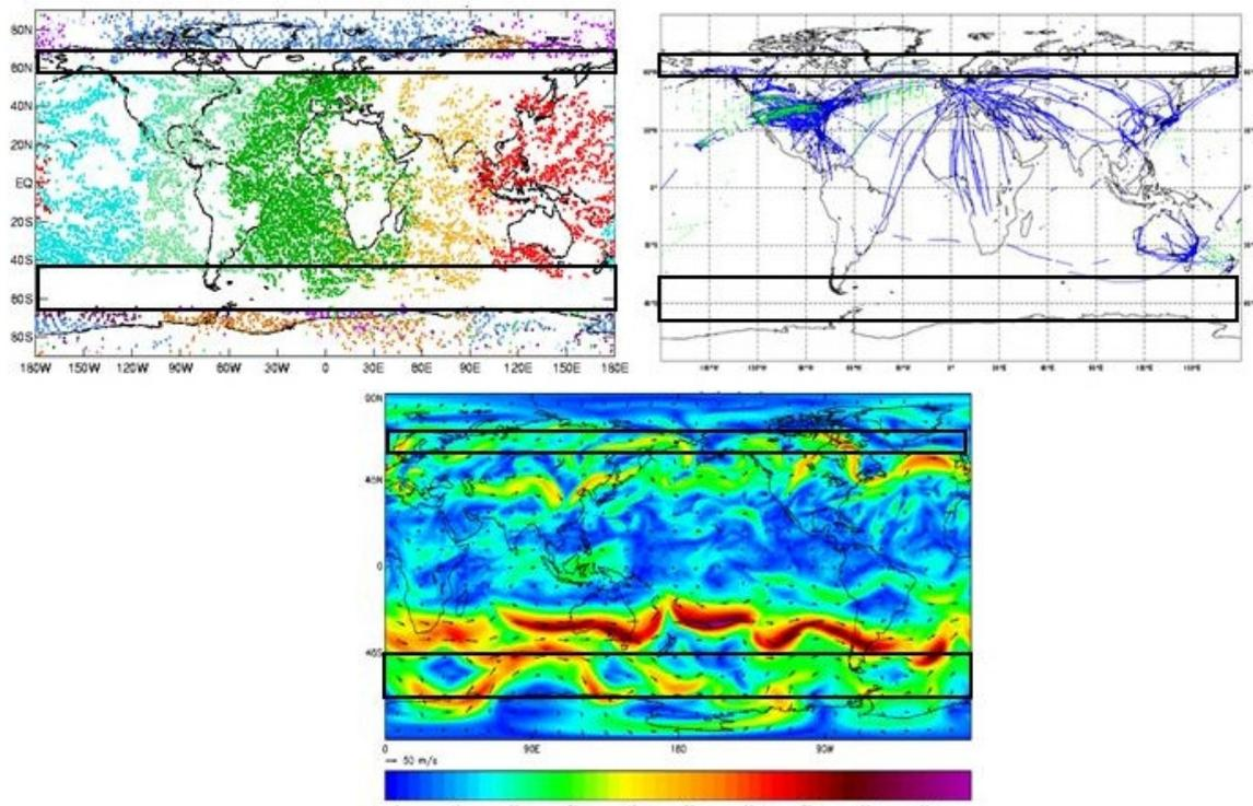
Figure 1: (top left) AMV coverage for 1500-2100 UTC on 8 July 2008, (top right) example aircraft coverage and (bottom) example 250 hPa model wind field showing the location of the jets. The boxes mark the main gaps in AMV coverage.
