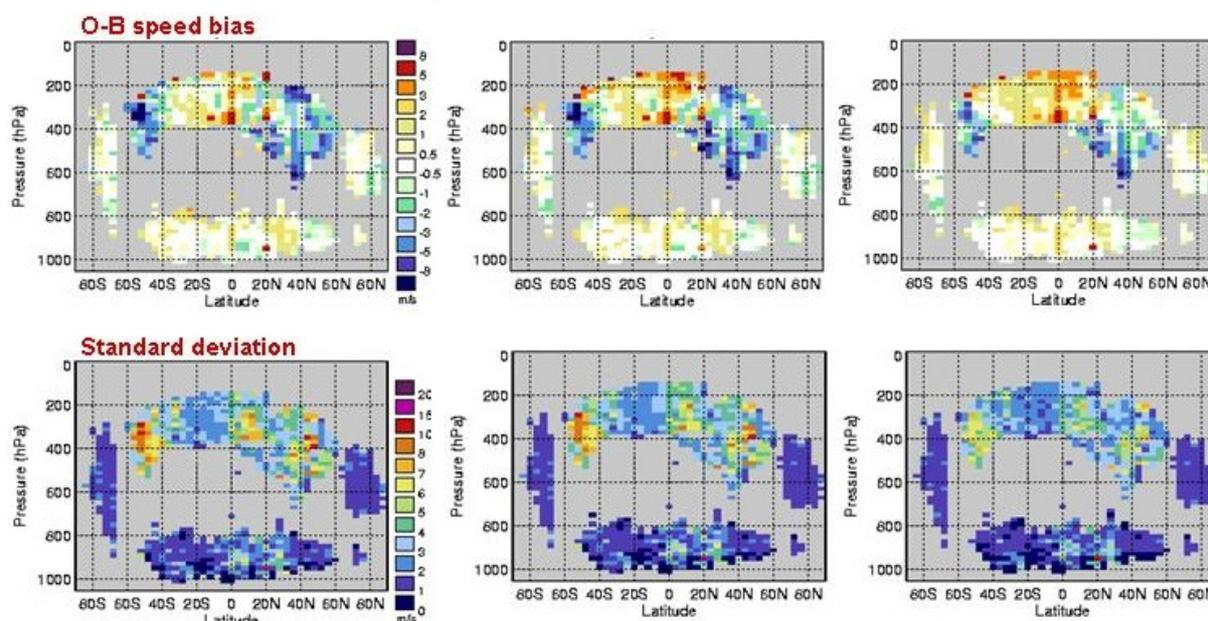
**Figure 8:** Preliminary results investigating the impact on O-B speed bias and standard deviation for all IR AMVs valid for 16 February 00 UTC run (2100-0300 UTC) when treated as: (left) single level (middle) 50 hPa fixed centred layer and (right) best-fit centred layer.
