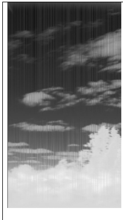
Figure 4. INO® microbolometer array from the UCL-MSSL test system of clouds (upper) and trees (lower). The 512-pixel array was scanned using a slow scanning mirror (3-4 minutes for a 1000 line scan). The sole artifact visible is the striping artifact.
