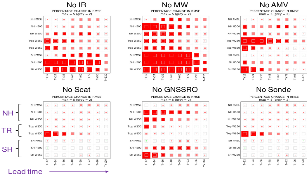
Figure 6: Percentage change in forecast RMS error (trial minus control) for various data denial trials verified against independent ECMWF analyses. Green squares indicate a positive impact from denying the observations (reduction in error) and red squares indicate a negative impact (increase in error). The size of the squares is scaled to the size of the RMS change with a maximum of 5% filling the square box.
